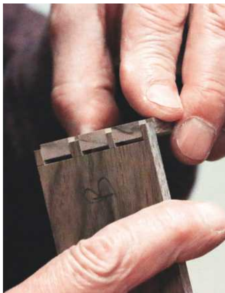
The result is a first-time perfect fit, achieved much quicker than when using normal methods
